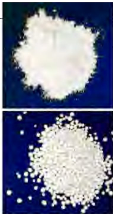
FIGURE 1. Fine potash powder is one example of an application that can benefit from particle enlargement
