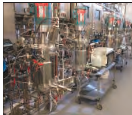
FIGURE 1. Pfenex evaluates top-performing strains in scaled-down bioreactors to optimize process parameters
