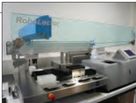
FIGURE 2. RoboLector, from m2p-labs, combines the ability to perform parallel fermentations with pipetting robotics
