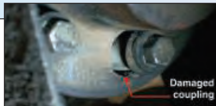
FIGURE 5. This case shows vibration results from resonance in a rotating equipment system. The phase difference between the horizontal and vertical components at the same bearing is close to zero. As seen in the photo, the hole in the coupling hub bolt became oblong-shaped due to persistent vibration damage. The time waveform for the axial direction shows periodic spacing with two humps at each peak. This situation can be addressed by modifying the piping and support systems
