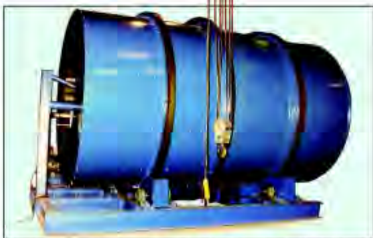
FIGURES 5 and 6. Wet agglomeration processes combine powder, liquid (usually water) and, if necessary, a binder, imparting shear to form agglomerates. Here, disc (left) and drum (right) agglomerators are shown
